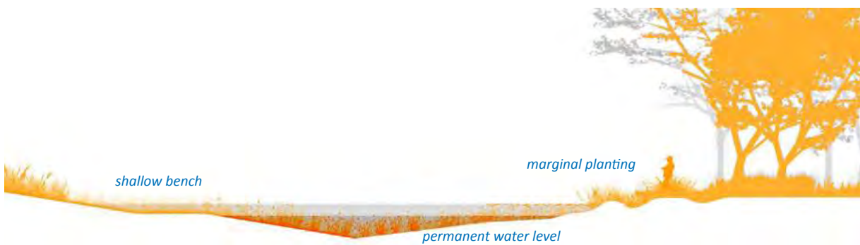
fig 10.2 - notional section through SUDS pond
