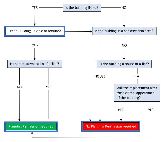
To avoid any misunderstandings as to what constitutes a "like for like" replacement, drawings are required to show full details of the replacement windows to be fitted.
