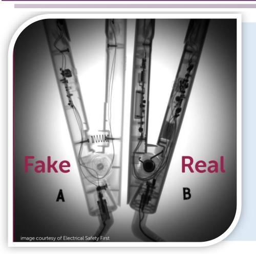
These x-ray images from Electrical Safety First show the difference between real and counterfeit straighteners
