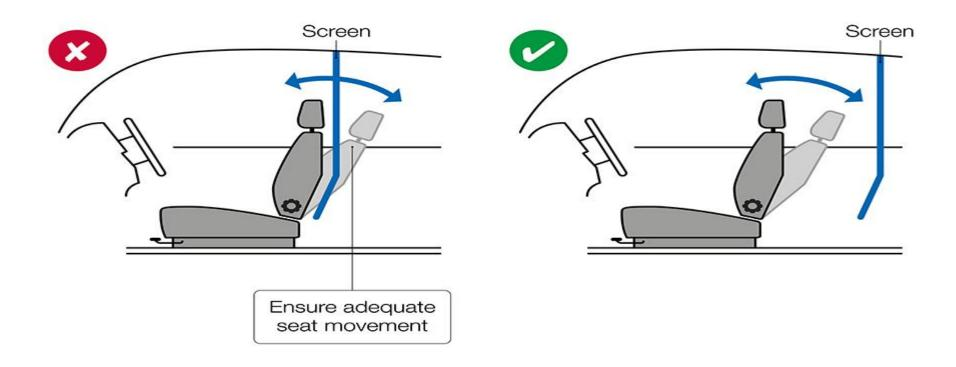
The fitting of the screen must not prevent the correct operation of seatbelts. The seatbelt webbing should not chafe against the screen or the fixing points, or adversely affect the operation of seatbelt pretensioners.
