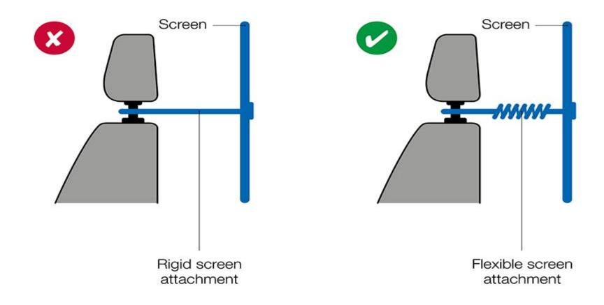
Figure 3b: avoid rigid fixings to head restraints
