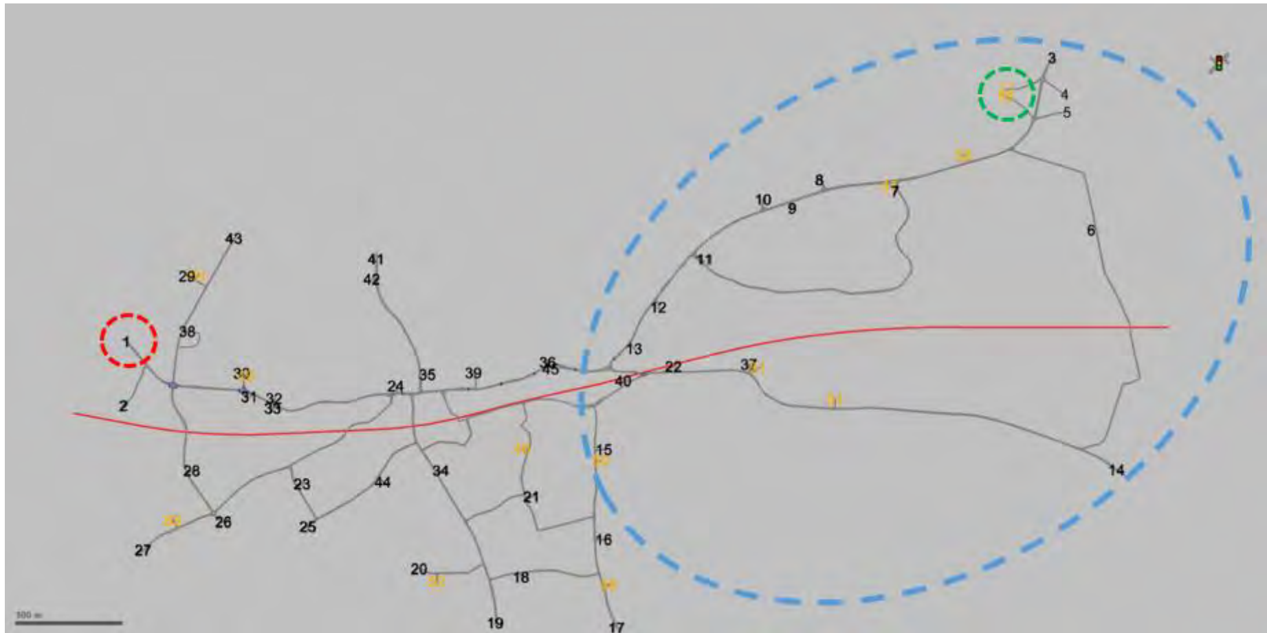
Figure 1. WFS Demand modification (blue = WFS catchment zones, red = original origin / destination zone, green = new WFS zones)
