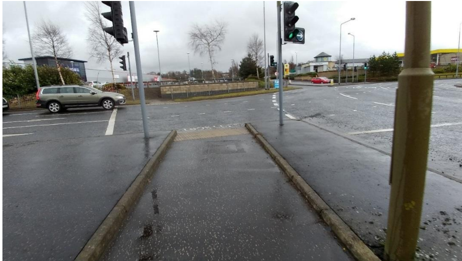
Image 6.28 - No Pedestrian Phase at roundabout
