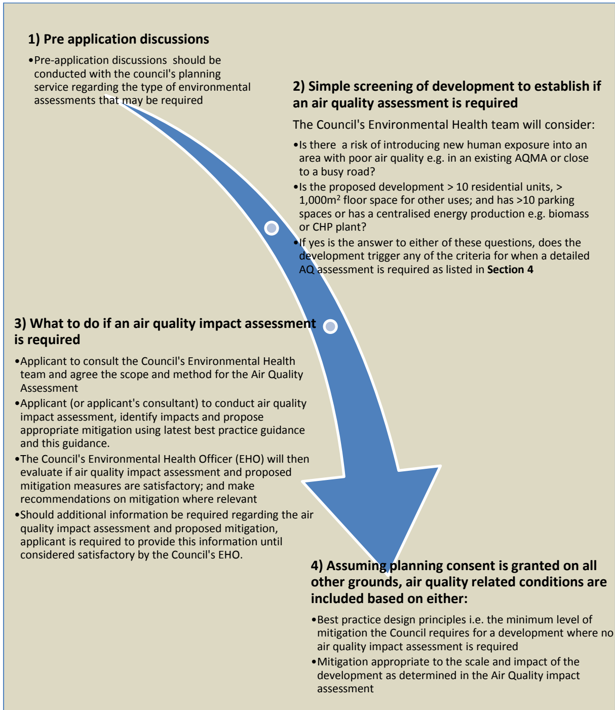
Figure 4: Steps explaining how air quality will be considered within the planning process
